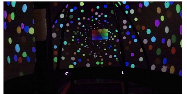
Figure 1. The roll dome is projected on the 6 m semicircular 180deg. Field of vision screen (eye-screen distance was 2.5 m). Subjects walk on the treadmill and are secured in a harness. In this experiment subjects were instructed to look at the rectangular shape. This shaped did not move during the experiment, the roll dome rotated counterclockwise.
